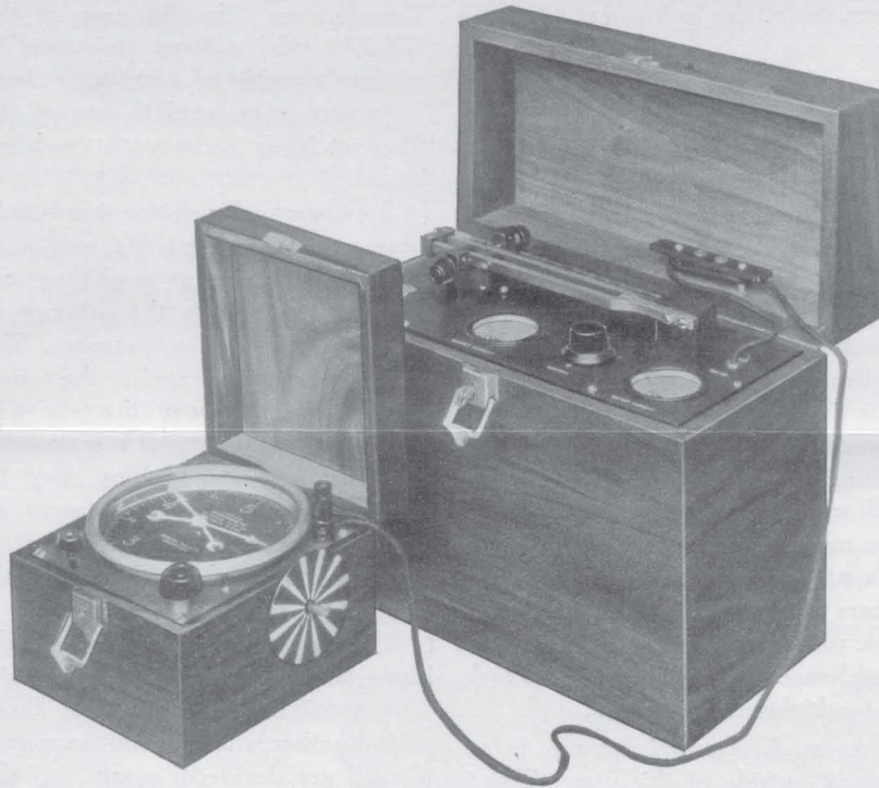
THE SYNCHRONOMETER WITH THE TYPE 467 SYNCHRONOUS DRIVING FORK
